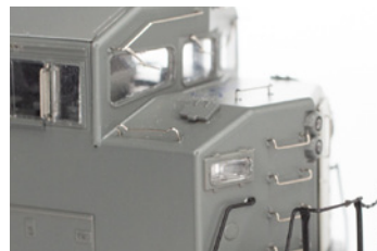
Standard nose bevel with large sand fill hatches
