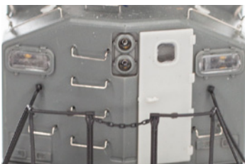
Small window nose door with front illuminated numberboards
