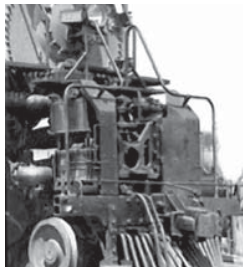
Boiler Tube with Widely Spaced Handrails
