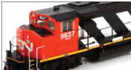
CN GP40-2W Lampshade ditch lights, snow shields, single rear headlight, no rear class lights or number boards
