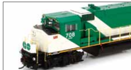
GO TRANSIT GP40-2W: Pilot mounted ditch lights. Rear vertical twin headlight, number boards, and class lights.
