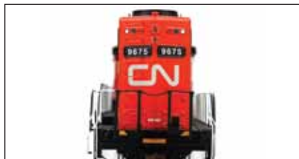
EX-GO TRANSIT CN GP40-2W: Lampshade ditch lights. Rear vertical twin headlight, number boards, and class lights.
