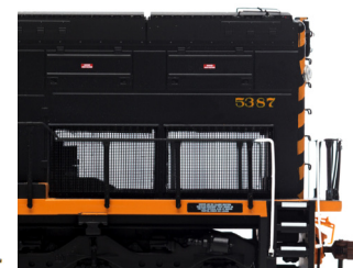
Gear tower moved, providing more visibly see-through grilles (SD40T-2 shown above).
