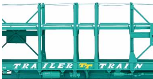
Updated F89FH including new lower deck, and side rails duplicating the Auto Rack mounts
