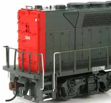
Steam Generator, Detailed Vents, and Flared Radiators
