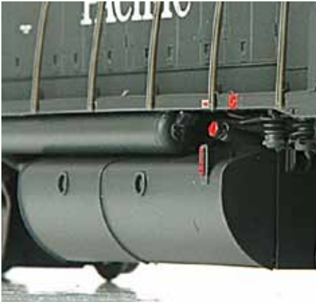
Split Diesel/Water Fuel Tank
