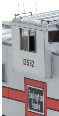
CB&Q & UP versions feature sliding cupola side windows
